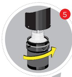
5 Place the sample bottle with clean Isopropyl alcohol in the Sample Cup Adapter and connect it to the instrument.
