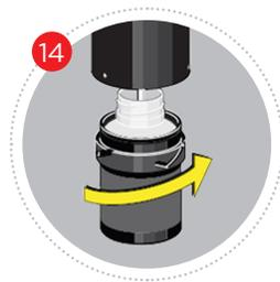
14 Place the sample bottle with clean MIL-5606 water in the Sample Cup Adapter and connect it to the instrument.
