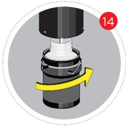
Place the sample bottle with clean DI water in the Sample Cup Adapter and connect it to the instrument.
