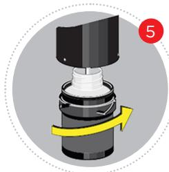
**5** Place the sample bottle with clean mineral spirits in the Sample Cup Adapter and connect it to the instrument.
